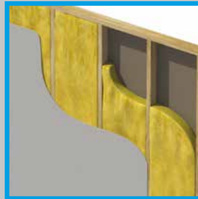
Internal wall - Insulating between timber joists
