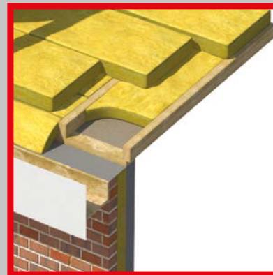
Lofts - Insulating between and over joists
