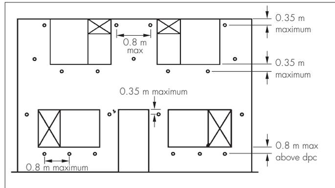
Figure 2 Typical drilling pattern — plain gable end
