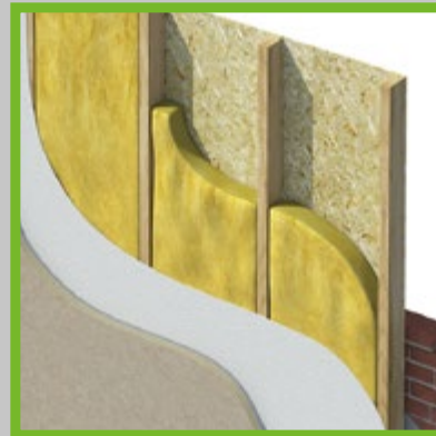
External Walls - Insulating between the timber studs
